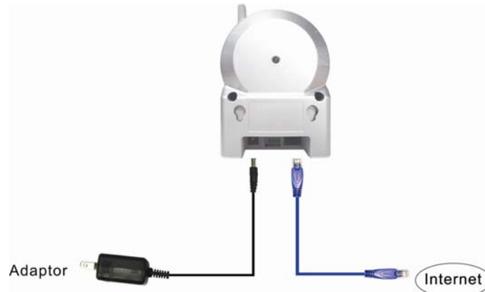
Figure 2-3: IP CAM connection diagram.
