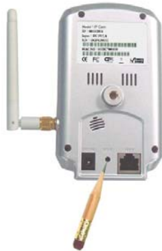
Figure 3-24: Stick on the reset button to set to the factory default
